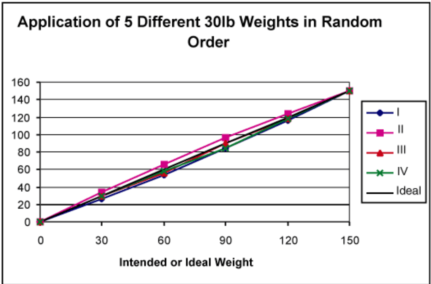
Figure 5: Sensor Output Variance Caused By Unequal Weights Applied In Random Sequence
